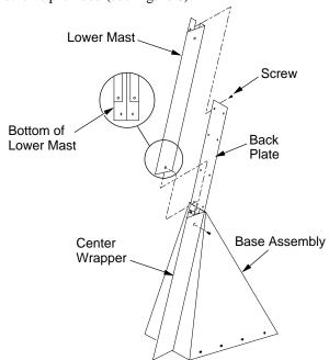
Figure 6 - Attaching Lower Mast
